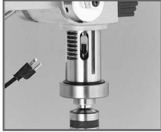
Figure 21. Inner and outer slots aligned.
